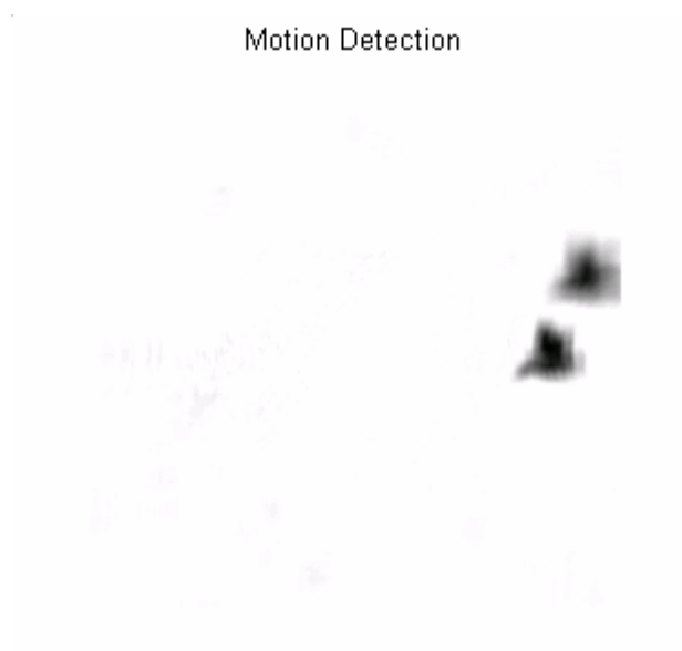
Fig. 4.60 Result of motion detection cells with 10 micro-saccades at time t=T_0+\delta
