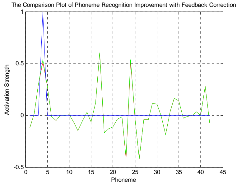
Figure 15. The comparison plots of phoneme recognition improvements with feedback connections: the blue line shows the desired results; the red line shows the results before adding sequence learning method; and the green line shows the final results with the feedback correction from the sequence learning block.
