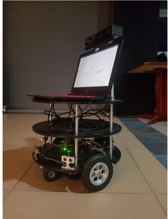
Figure 1 The Arlo mobile robot platform with the Kinect sensor used in experiments
