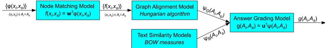
Figure 1: Pipeline model for scoring short-answer pairs.
