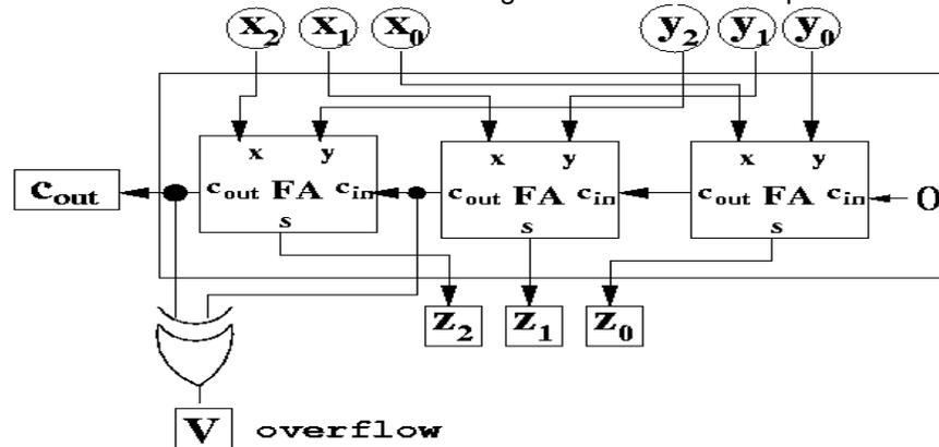
Notice the XOR gate at the bottom, which is exclusive-ORing the carry-in of the full adder of most significant bits to the carry-out.
